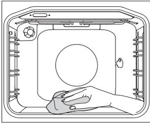
**1** Turn the COOKING SYSTEM SELECTOR KNOB to Aqua Clean. 2. Set the TEMPERATURE KNOB to 70 °C.
