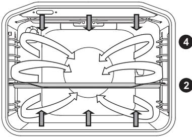
This function is used for baking of all types of pastry, for defrosting and for drying fruits and vegetables. Before placing the food into the preheated oven, wait for the light to go off for the first time. For best results, bake only on one shelf (level).
