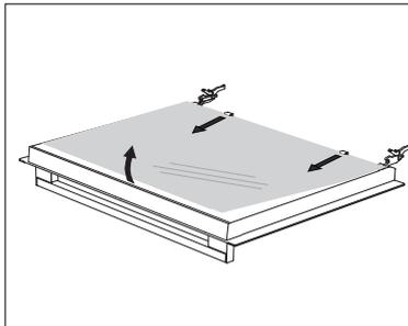
**3** Slightly lift the door glass and remove it from the clips on the bottom side of the door.
