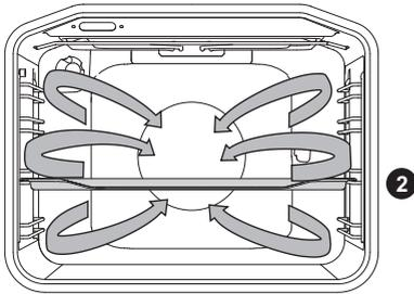
Round heater and the fan will operate. The fan installed in the back wall of the oven cavity, makes sure that hot air constantly circulates around the roast or pastry.
