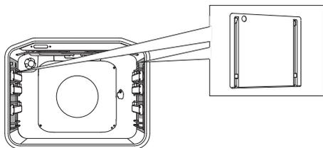
**CATALYTIC INSERTS** prevent the fat from sticking to sides of the oven cavity.
