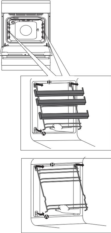
**A** Hold the guides by the bottom side and pull them towards the center of the oven cavity.
