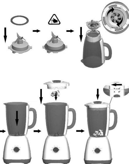
1. Install the jar sealing ring over the blending blade assembly.
