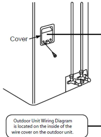
Outdoor Unit Wiring Diagram
