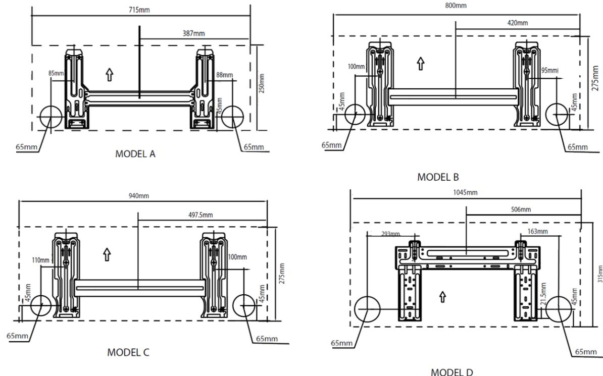
Picture 5: Recommended hole positions for gas pipes and electric wiring
