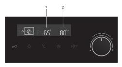
Turn the COOKING SYSTEM SELECTOR KNOB (hot air and lower heater). The symbol, oven cavity set temperature and meat probe set temperature will appear on the display unit. Press the START key.
