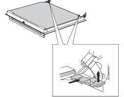
I Slightly lift the supports on the left and right side of the door (marking 1 on the support) and pull them away from the glass pane (marking 2 on the support).
