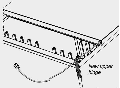
**12** Connect the control cable to the connector in the upper part of the drying cabinet. The control cable must be pulled through the hole as illustrated.
