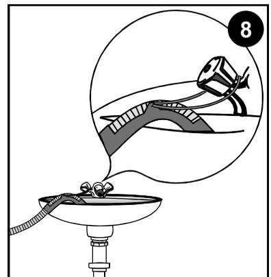
The end of the outlet hose should be raised from the floor by not more than 100 cm and not less than 60 cm. If the hose is positioned higher than recommended, the machine will not pump out the water.
