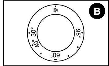
On the position marked with a snow flake, the heaters are switched off and you can select cold wash on all programmes. The duration of the programme is the same as if the heaters are on.
