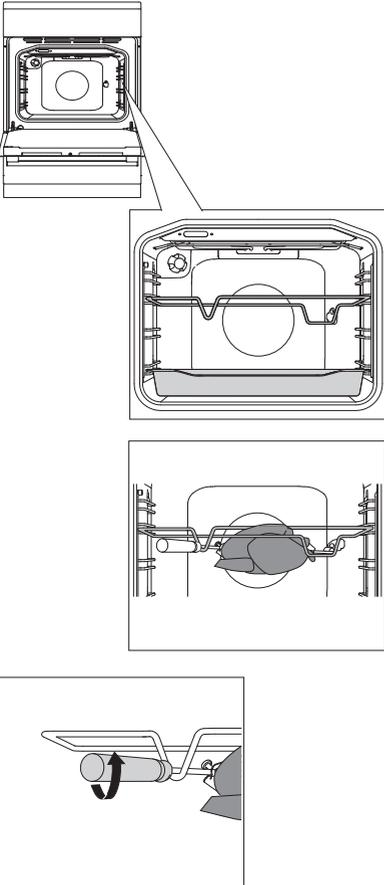
**1** Insert the skewer support into the 3rd guide from the bottom and place the deep tray into the bottom (1st) guide to serve as a drip tray.
