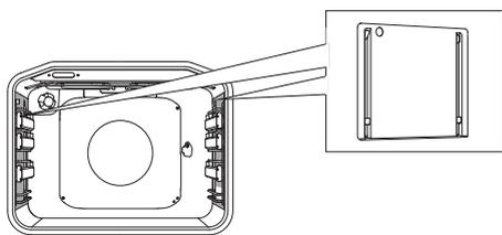
**CATALYTIC INSERTS** prevent the fat from sticking to sides of the oven cavity.
