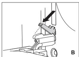
**B** With soft closing system, rotate the stoppers back by 90°.
