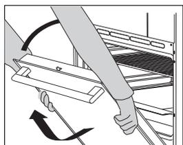
**3** Slowly close the door until the latches are aligned with the slots. Slightly lift the door and pull it out from both hinge slots on the appliance.
