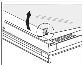
**1** Slightly lift the supports on the left and right side of the door (marking 1 on the support) and pull them away from the glass pane (marking 2 on the support).
