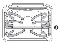
Round heater and the fan will operate. The fan installed in the back wall of the oven cavity makes sure the hot air constantly circulates around the roast or pastry.
