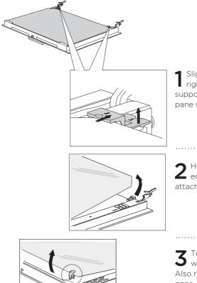
1 Slightly lift the supports on the left and right side of the door (marking 1 on the support) and pull them away from the glass pane (marking 2 on the support).
