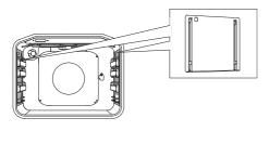
**CATALYTIC INSERTS** prevent the spraying fat from sticking to sides of the oven cavity.
