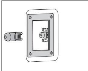
**2** Remove the halogen bulb.
