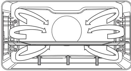
This is used for baking leavened but low-rising pastry and for preserving fruit and vegetables. Use the second guide from the bottom and a rather shallow baking tray to allow the hot air to circulate across the upper side of the dish.
