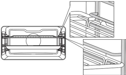
In case of wire guides, the tray should always be inserted into the groove between the two wire profiles.
