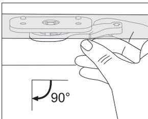
To reactivate the door lock, open the oven door and use your right-hand index finger to pull the lever towards you.
