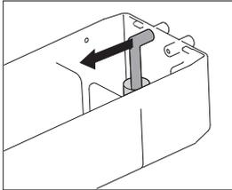
**2** Remove the inlet pipe from the pipe attachment.
