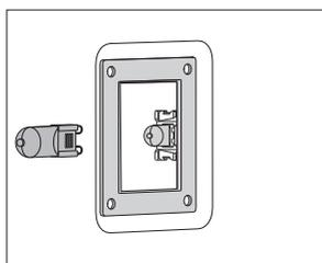
**2** Remove the halogen bulb.
