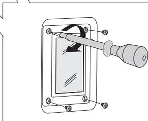
**1** Use a flat screwdriver to release the bulb cover and remove it.
