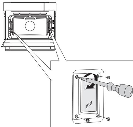
**1** Use a flat screwdriver to release the bulb cover and remove it.
