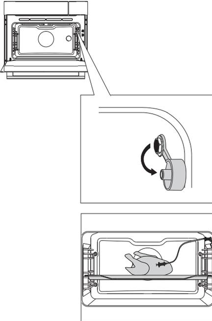
**1** Remove the cap (the socket is in the front upper corner of the oven right wall).
