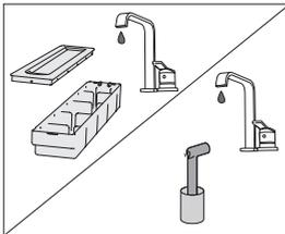
**3** Clean the inlet pipe with the filter foam under running water. Rinse the foam clean so that there are no visible impurities on it. Thus, you will make sure the appliance operates correctly and preserve the fresh flavour and smell of food.
