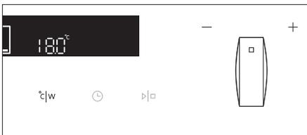
**2** Touch the TEMPERATURE KEY. Rotate the SETTINGS KNOB (-/+ ) and choose the desired temperature.
