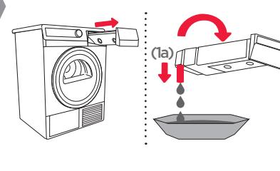
**1** Remove the condensate tank and turn it upside down above the sink or vessel to empty.
