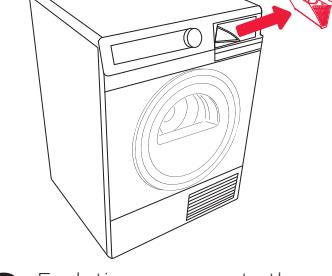
**2** Each time you empty the condensate tank, **clean the steam generator tank filter**.
