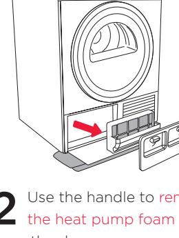
**2** Use the handle to **remove the heat pump foam filter** from the dryer.
