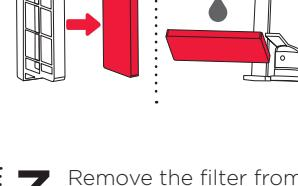
**3** Remove the filter from its handle and use a damp cloth to clean the housing.
