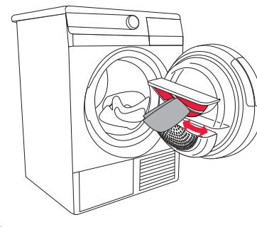
**2** **Scrape the filter cover to remove the layer of lint and threads.**
