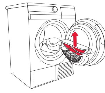
**1** Open the filter cover, and **remove** the net filter.
