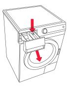
To remove the dispenser tray from the housing, press the small lever.
