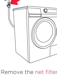
**1** Remove the net filter from the inlet hose.
