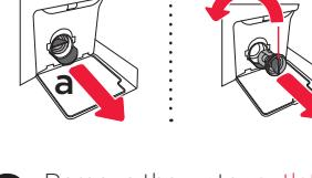
**2** Remove the water outlet funnel (a) before cleaning the filter. Rotate the filter slowly in the counter-clockwise direction (b). Remove the filter to allow the water to slowly drain.
