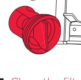
**3** Clean the filter under running water and replace it.
