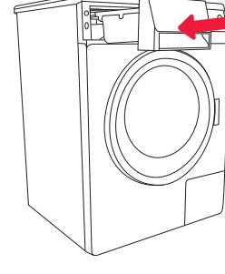
**1** Before replacing the dispense tray, also clean the rinsing area.
