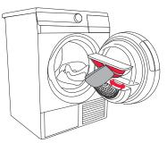
Scrape the filter cover to remove the layer of lint and threads.
