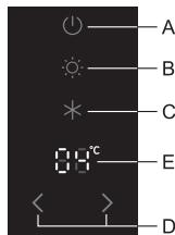
**Switching the appliance on:** Switch on the appliance by briefly pressing the key **A**.
