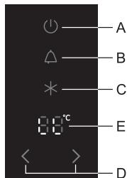
Use this function if you do not wish to manually adjust the appliance settings. To activate, press and hold the **B** key (for three seconds); **LL** will appear on the display **E**. This will lock all keys except **B**. To deactivate the safety lock, press the **B** key and hold it for three seconds.
