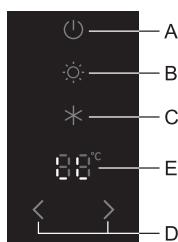
Use this function if you do not wish to manually adjust the appliance settings. To activate, press and hold the **B** key (for three seconds); **LL** will appear on the display **E**. This will lock all keys except **B**. To deactivate the safety lock, press the **B** key and hold it for three seconds.
