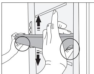
The height of the door bins can be adjusted without having to remove the bins from the appliance. Simply pull the two levers on each side of the bin towards you and slide the bin up or down.
