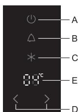
If the temperature inside the appliance is too high, acoustic alarm will be activated (**intermittent tone**) and the **B** key will flash.
