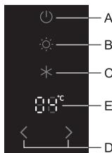
If the temperature inside the appliance is too high, acoustic alarm will be activated (**intermittent tone**) and the temperature display will flash.
