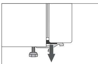
Spacers are fitted on the corners of the doors.
