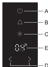
**Switching the appliance on:** Switch on the appliance by briefly pressing the key **A**.
