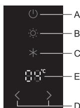
**VitaLED:** press the **B** key to switch the VitaLED on or off. When the VitaLED is switched on, the **B** key will be lit up. When the VitaLED function is activated, the orange LED lighting in the fruit and vegetable bin will be switched on. In case of a power outage, the VitaLED function will not remain activated. VitaLED prolongs the freshness of food and allows it to retain the flavour and the nutrients. Use it only when necessary as it increases power consumption.
