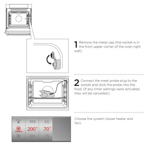
Preset temperature and probe temperature will be displayed. Touch the START key.
