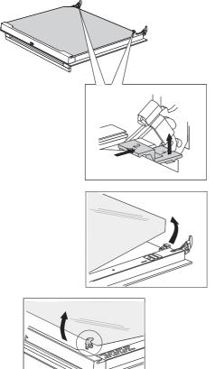
Slightly lift the supports on the left and right side of the door (marking 1 on the support) and pull them away from the glass pane (marking 2 on the support).
