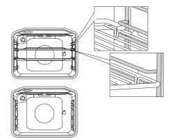
With telescopic extendible guides, first pull out the guides of one level and place the grid or the baking tray onto them. Then, push them in with your hand as far as they will go.
