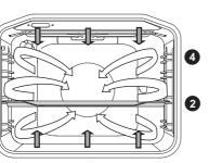
It is used for baking of all types of pastry, for defrosting, and for drying fruit and vegetables. Before placing the food into the preheated oven, wait for the light to go off for the first time. For best results, only bake on one shelf (level).
