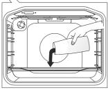
**2** Pour 0.6 I water into the glass tray and place it into the lower guide.
