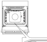
Turn the COOKING SYSTEM SELECTOR KNOB to Aqua Clean. 2. Set the TEMPERATURE KNOB to 70 °C.
