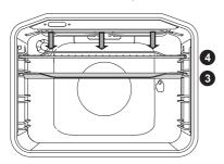
When grilling food with the large grill, the upper heater and the grill heater fitted on the ceiling of the oven cavity will operate.
