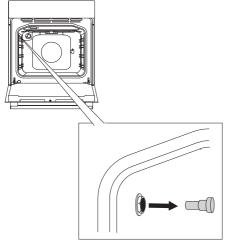
Remove the metal cap (the socket is located in the front upper corner of the oven right wall).
