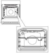
Insert the skewer support into the 3rd guide from the bottom and place the deep tray into the bottom (1st) guide to serve as a drip tray.
