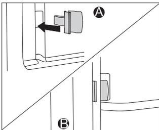
When installing fully extendible guides with catalytic inserts, insert one end of the supplied snap locks into the openings at the bottom of the oven cavity wall and insert the other end of the snap locks into the guides.
