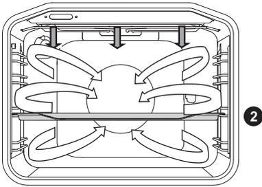
In this operating mode, the grill heater and the fan operate simultaneously. Suitable for grilling meat, fish, and vegetables.
