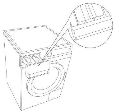
Washing machine is equipped with the dispenser left gate, so you may pour liquid detergent also into the central compartment (depending on model). If you use powder detergent the gate is lifted up, and in case of liquid detergent it is slid down.
