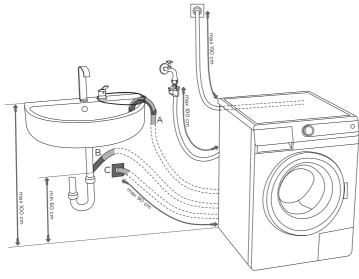
Outlet hose can be led into a wash basin or a bathtub. Use a string to attach the hose to the opening in the elbow support to prevent it from slipping to the floor.
