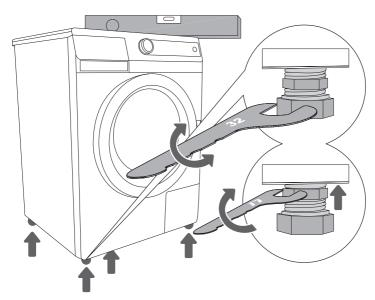
Put the appliance in horizontal position by turning the adjustable legs. The legs are adjustable up to +/-1 cm.
