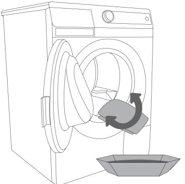
Clean the washing machine drum before using the appliance for the first time. Use a damp cloth and a mild cleaning agent, or run the self-cleaning program (SterilTub).
