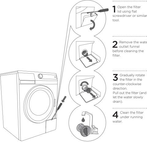
Open the filter lid using flat screwdriver or similar
