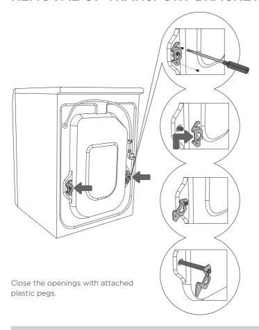
Move the pipes. Loosen screws at the rear of the machine
