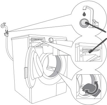
Clean the water inlet hose screen frequently under running water.
