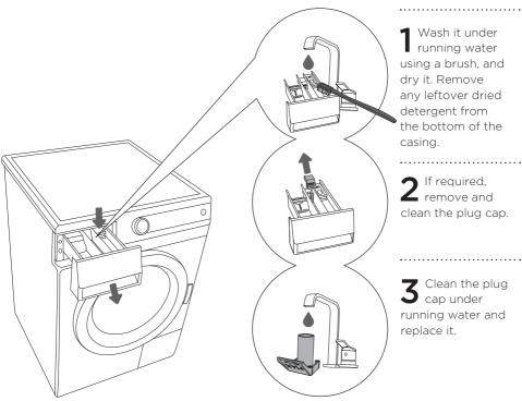
Wash it under running water using a brush, and dry it. Remove any leftover dried detergent from the bottom of the
