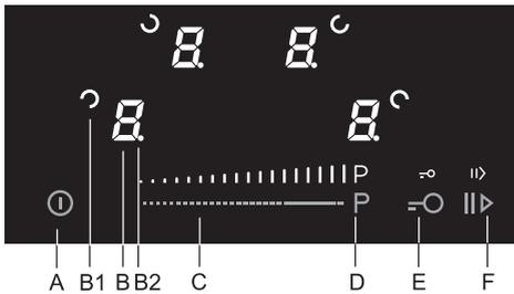
To activate the automatic rapid heating, select the desired cooking zone by touching the (B) key. Then, set the desired cooking power on the slider (C). Hold a finger on the selected level for around 3 seconds until you hear a beep and "A" appears on the display unit (B).
