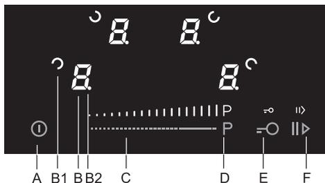
Touch the on/off sensor key (A) and hold it for at least 1 second. The cooking hob will be activated and the display units will light up.
