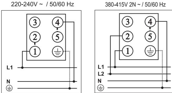
The appliance is designed for two-phase connection; it can also be connected to a single phase.
