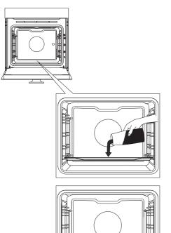
Turn the COOKING SYSTEM SELECTOR KNOB to Aqua Clean. An icon will be displayed along with the PRESET TEMPERATURE and the time of 30 minutes.
