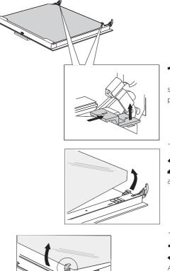
**1** Slightly lift the supports on the left and right side of the door (marking 1 on the support) and pull them away from the glass pane (marking 2 on the support).
