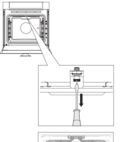
**1** To remove the heater, undo the screw located at the front of the oven cavity ceiling.
