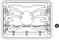
This is used for baking leavened but lowrising pastry and for preserving fruit and vegetables. Use the second guide from the bottom and a rather shallow baking tray to allow the hot air to circulate across the upper side of the dish.
