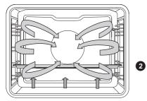
The bottom heater, the round heater, and the hot air fan will operate. Suitable for baking pizzas, apple pies, and fruitcakes.
