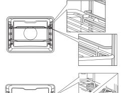
With telescopic extendible guides, first pull out the guides of one level and place the grid or the baking tray onto them. Then, push them in with your hand as far as they will go.
