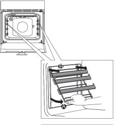
**A** Hold the guides by the bottom side and pull them towards the center of the oven cavity.
