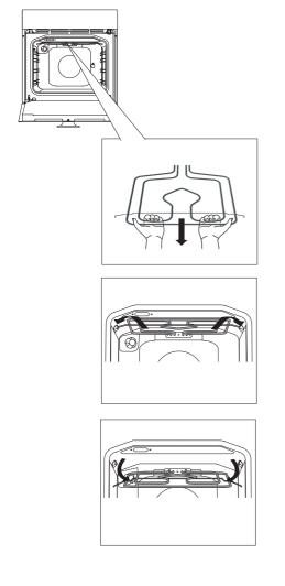
Pull the heater until the cross bar is released from the supports on the left and right hand side of the oven cavity.
