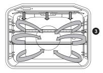
In the automatic meat cooking mode (Auto Roast), the upper heater will operate in combination with the round heater. It is used for roasting all types of meat.
