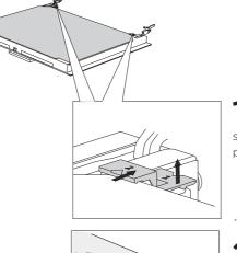
1 Slightly lift the supports on the left and right side of the door (marking 1 on the support) and pull them away from the glass pane (marking 2 on the support).
