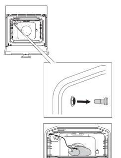
Remove the metal cap (the socket is located in the front upper corner of the oven right wall).
