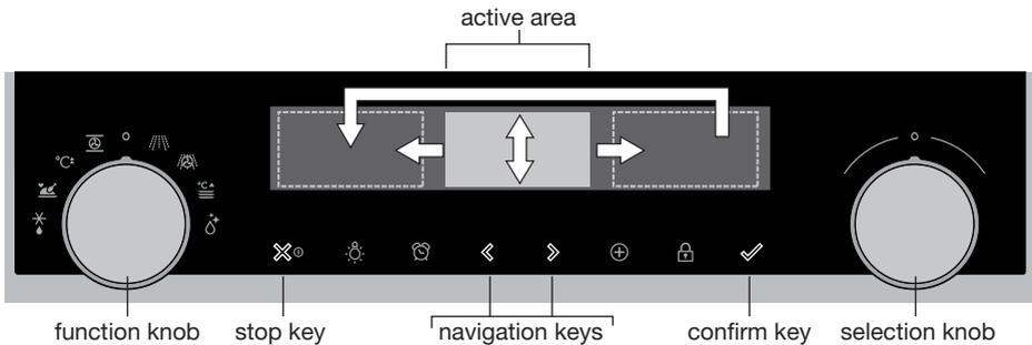
By turning the function knob away from the 0-position, the icon of the chosen main function is lit. The display will show the icon and name of the activated function for about 1,5 seconds. Next you will see the chosen main function and sub-function at the top of the display in the feedback bar. Also the function settings mode will become active (grey background). In this activated area you can select your settings using the selection knob.
