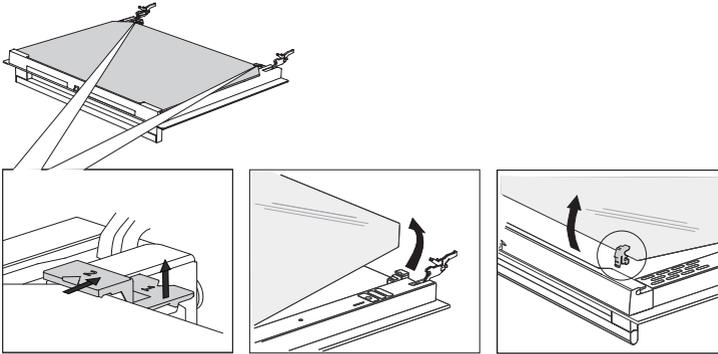
To replace the glass pane, observe the reverse order. The markings (semicircle) on the door and the glass pane should overlap.
