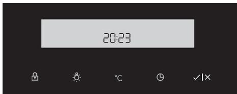
Confirm by pressing START/ STOP. If nothing is pressed within the next three seconds, the setting will be stored automatically.
