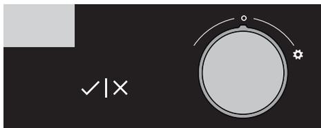
Rotate the SETTINGS KNOB (-/+ ) and first set the minutes; then, the cursor will switch to hours. After three seconds, the settings will be saved.
