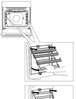
**A** Hold the guides by the bottom side and pull them towards the center of the oven cavity.
