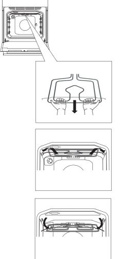
Pull the heater until the cross bar is released from the supports on the left and right hand side of the oven cavity.
