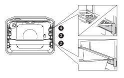
With telescopic extendible guides, first pull out the guides of one level and place the grid or the baking tray onto them. Then, push them in with your hand as far as they will go.
