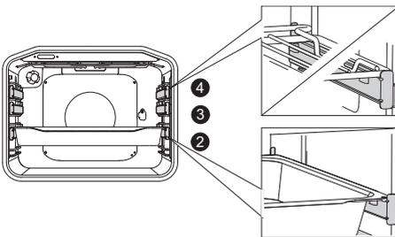
💡 Close the oven door when the telescopic guides are retracted all the way into the oven.
