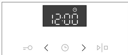
**1** Set the clock by touching the < or > keys, and confirm the setting by touching the ☹ key.
