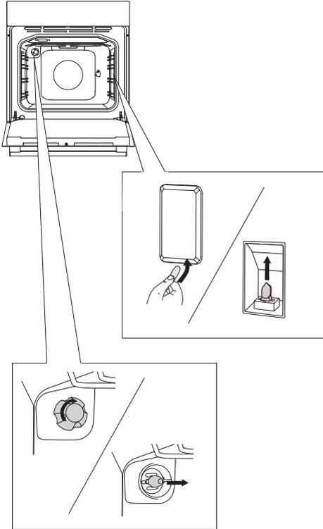
Use a flat screwdriver to release the bulb cover and remove it. Remove the bulb.
