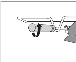
**1** Insert the skewer support into the 3rd guide from the bottom and place the deep tray into the bottom (1st) guide to serve as a drip tray.
