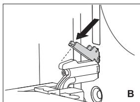
**B** If the appliance is fitted with the GentleClose system, flip the door latches back to a 90° angle (Figure 2).
