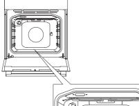
Turn the COOKING SYSTEM SELECTOR KNOB to Aqua Clean. 2. Set the TEMPERATURE KNOB to 70 °C.
