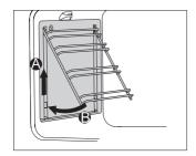
2 Hang the inserts with guides attached using the holes provided, and pull upwards.
