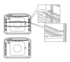
The grid or the tray should always be inserted into the groove between the two wire profiles.
