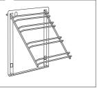
Mount the guides onto the catalytic insert.
