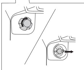
Undo the bulb cover and remove the bulb.
