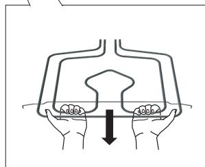
Pull the heater until the cross bar is released from the supports on the left and right hand side of the oven cavity.
