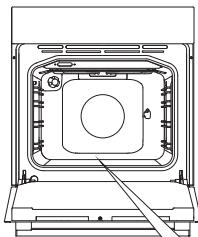
**1** Turn the COOKING SYSTEM SELECTOR KNOB to Aqua Clean. 2. Set the TEMPERATURE KNOB to 70 °C.
