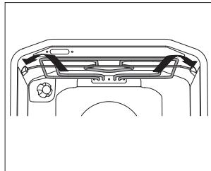
Never use the heater when folded/lowered. After cleaning, observe the same procedure in the reverse order to push back the heater until the cross bar snaps back into place.
