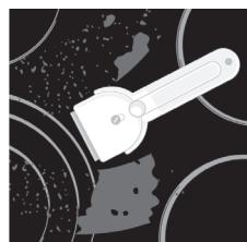
Remove stubborn and burnt residues with a scraper. Be careful when handling the scraper to prevent injury.
