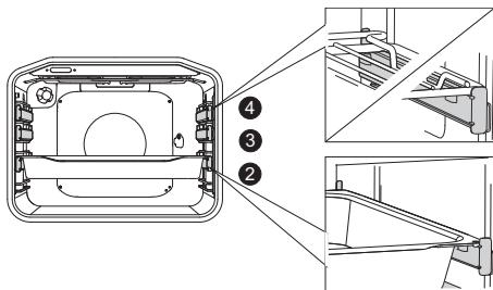
With telescopic extendible guides, first pull out the guides of one level and place the grid or the baking tray onto them. Then, push them in with your hand as far as they will go.
