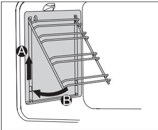
**2** Hang the inserts with guides attached using the holes provided, and pull upwards.
