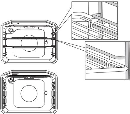
The grid or the tray should always be inserted into the groove between the two wire profiles.
