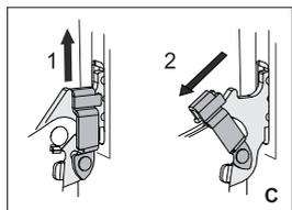
**C** If the appliance is fitted with the GentleClose system, slightly lift the door latches and pull them towards you.
