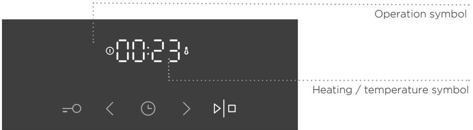
While the oven is heating up, the temperature symbol will flash. When the oven reaches the set temperature, the symbol will light up and a short beep will be sounded.
