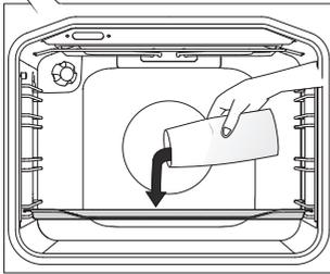
**2** Pour 0.6 l water into the deep baking tray and place it in the lower guide
