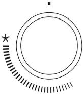
On the knobs, heating power levels are indicated with thick and thin markings. Rotate the knob past the asterisk (\*) position and the thick markings to the thin markings position and back. Operating position is within the range indicated by the markings. Settings between (\*) and (■) are not recommended. In this range, the flame is unstable and may be extinguished.
