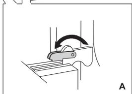
**2** **A** Rotate the stoppers all the way back (in case of conventional closing).
