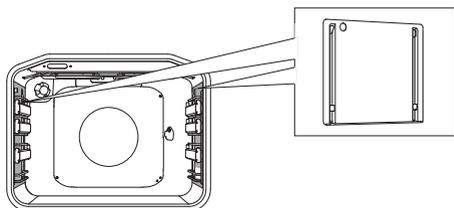
**CATALYTIC INSERTS** prevent the spraying fat from sticking to sides of the oven cavity.
