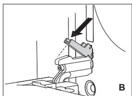
**B** With soft closing system, rotate the stoppers back by 90°.
