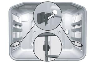
When installing telescopic retractable guides (which can be pulled out completely) and the easy-clean inserts, insert the supplied clips into the lower openings on the oven interior walls, and insert the guides into these clips. The clips are intended for securing the guides.
