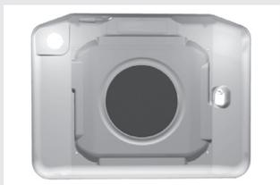
The fat filter installed on the back oven interior wall protects the fan, round heater, and the oven from impurity, particularly spattering fat. When cooking meat, we recommend using the fat filter. When baking pastry, always remove the filter! If the filter is installed when baking pastry or cakes, the results can be quite poor.
