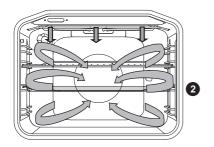
In the automatic meat cooking mode (Auto Roast), the upper heater will operate in combination with the round heater. It is used for roasting all types of meat.
