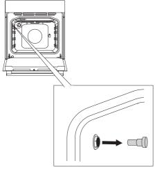
Remove the metal cap (the socket is located in the front upper corner of the oven right wall).
