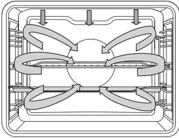
In the Auto Roast mode, the upper heater will operate in combination with the grill heater and the round heater. It is used for roasting all types of meat.
