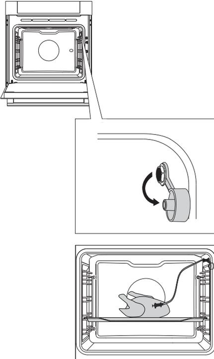
**1** Remove the metal cap (the socket is in the front upper corner of the oven right wall).
