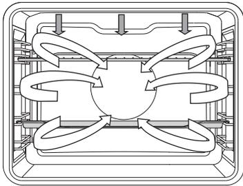
In this operating mode, the grill heater and the fan operate simultaneously. Suitable for grilling meat, fish, and vegetables.
