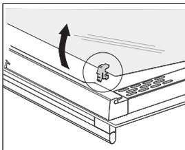
**3** To remove the third glass pane (only with some models), lift and remove it. Also remove the rubber seals on the glass pane.
