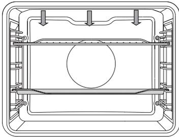
When grilling food with the **large grill**, the upper heater and the grill heater fitted on the ceiling of the oven cavity will operate.
