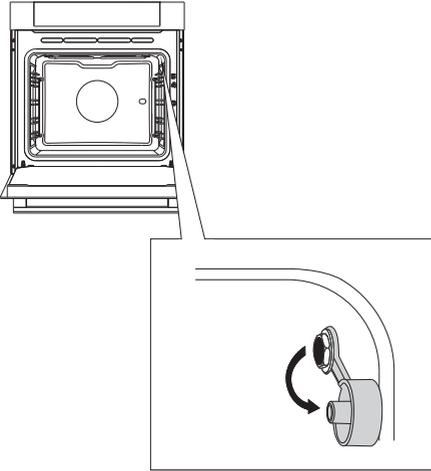
**1** Remove the metal cap (the socket is in the front upper corner of the oven right wall).
