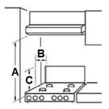
Overhead clearances—(Measurement A) Range hoods and exaust fans shall be installed in accordance with the manufacturer's relevant instructions. However, in no case shall the clearance between the highest part of the hob of the gas cooking appliance and a range hood be less than 600 mm or, for an overhead exhaust fan, 750 mm.
