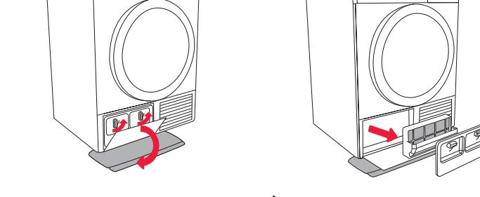
**1** Place an absorbent cloth on the floor in front of the dryer.
