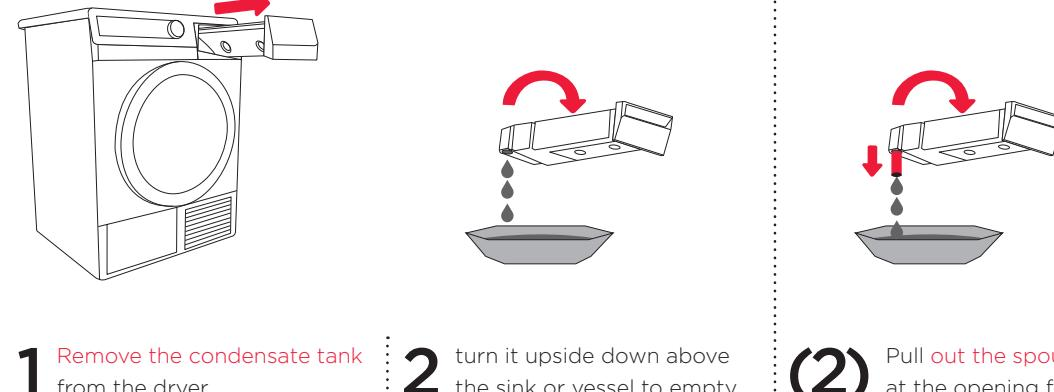
**1** Remove the condensate tank from the dryer.
