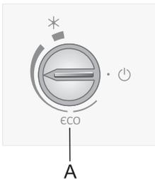
**To switch on:** rotate the thermostat knob **A** clockwise towards **the thicker end of the sign.**
