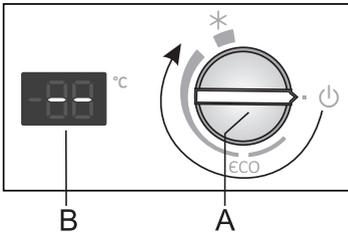
**Switching on:** To switch on: rotate the **A** dial clockwise.
