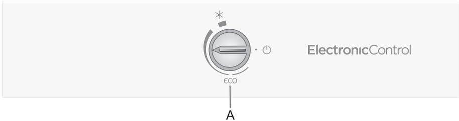
A Knob for temperature settings, switching the appliance on/off, and activating the super freeze function
