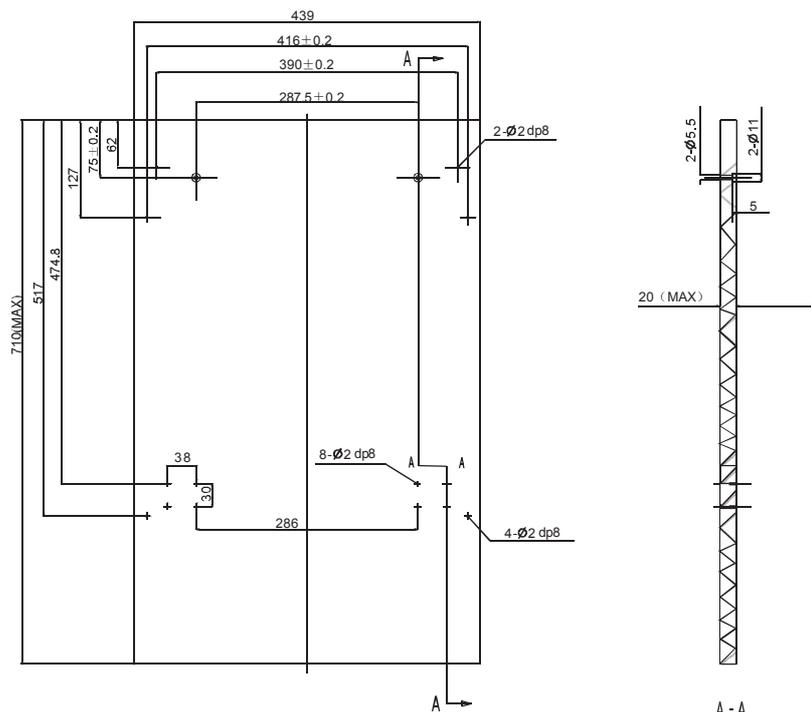
2 Install the hook on the aesthetic wooden panel and put the hook into the slot of the outer door of dishwasher(see figure 4a). After positioning of the panel , fix the panel onto the outer door by screws and bolts(See figure 4b) .
