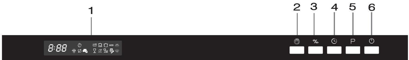
1. Display screen: to show the error code, delay time etc.
