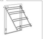
Mount the guides onto the catalytic insert.
