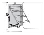
Hang the inserts with guides attached using the holes provided, and pull upwards.
