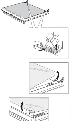
**1** Slightly lift the supports on the left and right side of the door (marking 1 on the support) and pull them away from the glass pane (marking 2 on the support).
