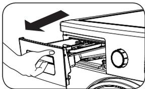
Your detergents may deposit residue in the detergent drawer and housing of the detergent drawer over time. To clean the residue, disassemble the detergent drawer at regular intervals. It is recommended that you clean your detergent drawer every 2 months.
