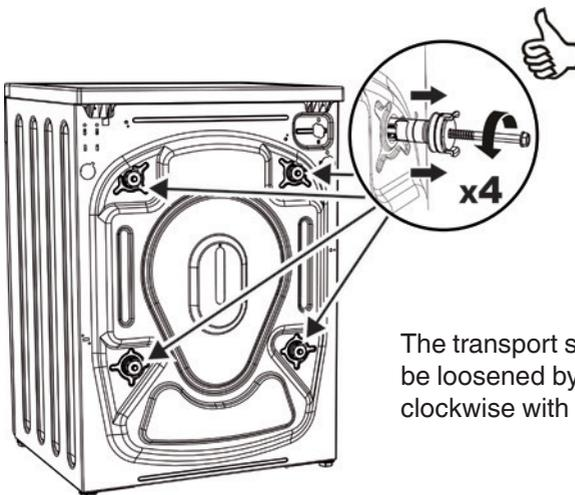
The transport safety screws should be loosened by rotating them counter clockwise with an appropriate wrench.
