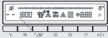
If you have missed the washing water temperature you wanted, you can return to the intended temperature by continuously pressing the washing water temperature adjustment button.
