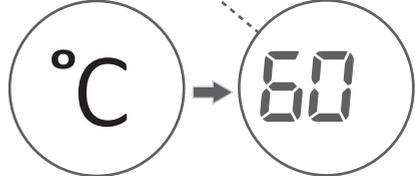
You can gradually decrease the washing water temperature between the maximum temperature and cold washing (--) by pressing the washing water temperature adjustment button.
