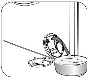
Your machine contains a filter system that prevents thread or fluff left over from your laundry and other small materials from entering the pump during the discharge operation after a completed wash cycle. This is to protect and prolong the life of the pump. It is recommended that you clean your pump filter once every 2 months.
