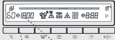
Whenever you select a new programme, the maximum washing water temperature is shown on the washing water temperature display.
