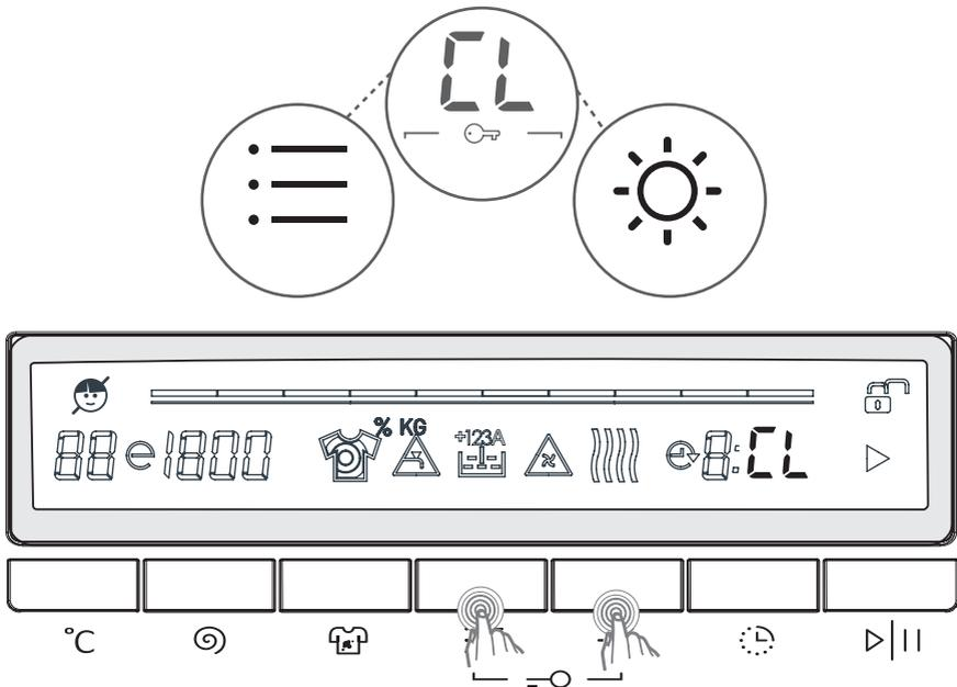
“CL” symbol will flash on the electronic display when activated.
