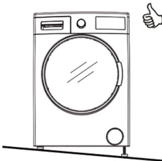
You can adjust the balance of your machine by means of the adjustable feet.
