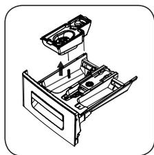
For the cleaning and maintenance of the liquid detergent level apparatus, remove the apparatus from its location as shown in the picture and thoroughly clean the detergent residues. Put the apparatus back into its place. Make sure no residues are left inside.
