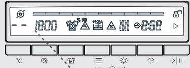
If you have missed the washing water temperature you wanted, you can return to the intended temperature by continuously pressing the washing water temperature adjustment button.
