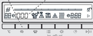
You can gradually reduce the revolution speed between cancel spinning (-) options through to the maximum spin revolution of the programme selected by pressing the revolution speed setting button.
