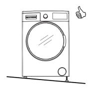
To ensure silent and vibration-free operation of your machine, it should be deployed on a non-sliding and firm ground.
