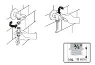
**Note:** Use only the new water inlet hose coming with your machine when making the water inlet connections. Never use old, used or damaged water inlet hoses.
