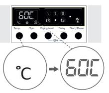
You can gradually decrease the washing water temperature between the maximum temperature and cold washing (--) by pressing the washing water temperature adjustment button.
