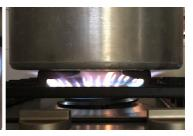
In contrast to propane gas, conversion to butane gas will result in a more yellow flame pattern (yellow tipping). Yellow tipping is customary and safe and has no negative impact on combustion, use etc.
