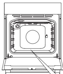
**1** Okrenite DUGME ZA IZBOR SISTEMA PEĆENJA na Aqua clean. DUGME ZA IZBOR TEMPERATURE postavite na 70°
