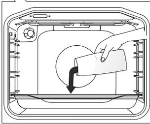
**2** Pour 0.6 l water into the glass tray and place it into the lower guide.
