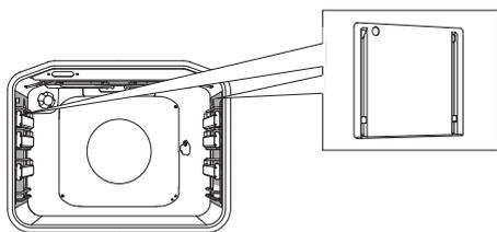
**CATALYTIC INSERTS** prevent the spraying fat from sticking to sides of the oven cavity.
