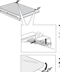
Slightly lift the supports on the left and right side of the door (marking 1 on the support) and pull them away from the glass pane (marking 2 on the support).
