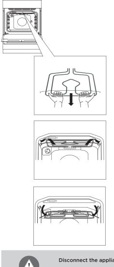
Pull the heater until the cross bar is released from the supports on the left and right hand side of the oven cavity.
