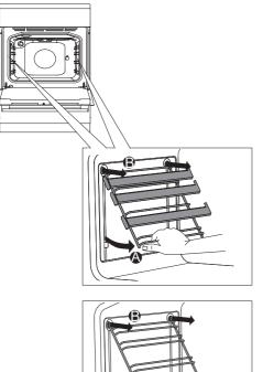
**A** Hold the guides by the bottom side and pull them towards the center of the oven cavity.
