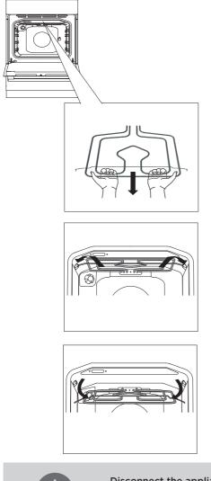
Pull the heater until the cross bar is released from the supports on the left and right hand side of the oven cavity.
