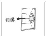
2 Remove the halogen bulb.
