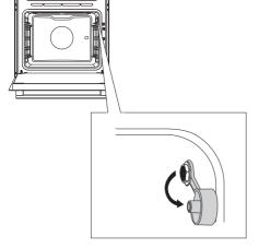
Remove the metal cap (the socket is in the front upper corner of the oven right wall).
