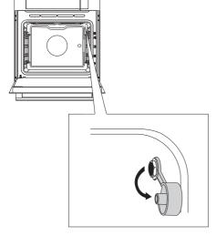
Remove the cap (the socket is in the front upper corner of the oven right wall).
