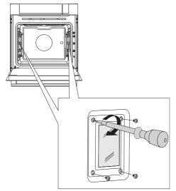
1 Use a flat screwdriver to release the bulb cover and remove it.
