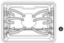
Round heater and the fan will operate. The fan installed in the back wall of the oven cavity makes sure the hot air constantly circulates around the roast or pastry.
