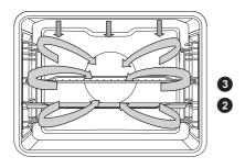
In the Auto Roast mode, the upper heater will operate in combination with the grill heater and the round heater. It is used for roasting all types of meat.
