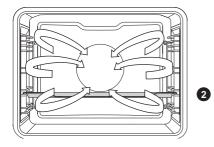
Water from the steam generator enters the oven cavity in the form of steam.
