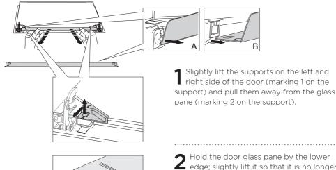
Hold the door glass pane by the lower dedge; slightly lift it so that it is no longer attached to the support; and remove it.
