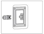
**?** Remove the halogen bulb.
